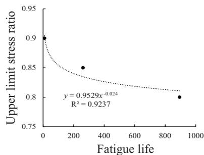
Fig. 4. Relationship curve between different upper limit stress and fatigue life
