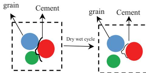
Fig. 7. Particle change after dry wet cycle
