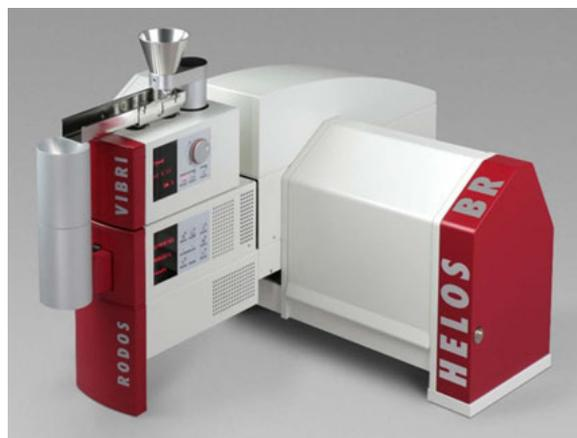
Fig. 2. The set for dry measurements: HELOS diffractometer, RODOS dispersant, VIBRI feeder [37]
