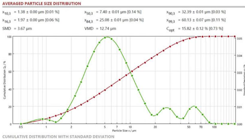
Fig. 5. The average particle size distribution by Laser Diffractometer for soil No. 1 ( $LOI_T = 7.71\%$ )
