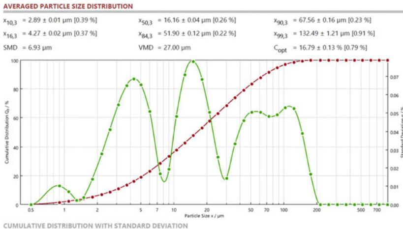
Fig. 6. The average particle size distribution by Laser Diffractometer for soil No. 2 ( $LOI_T = 48.71\%$ )
