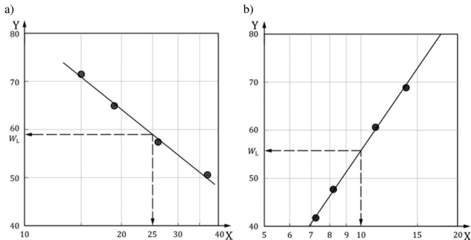
Fig. 3. The example of a the liquid limit test result based to the rules of the standard [35] from:
