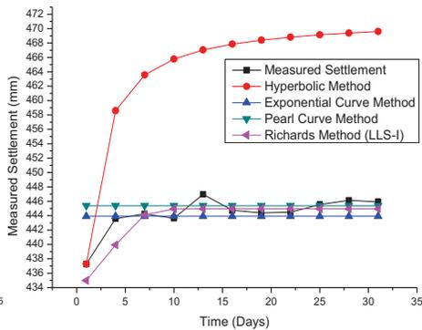
Fig: 4. Curve fitting of Observation section K10+900-1
