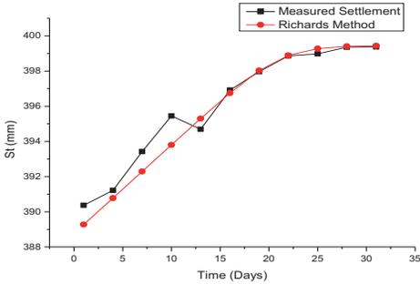
Fig. 2. Measured and predicted settlement values for section K10+900-1
