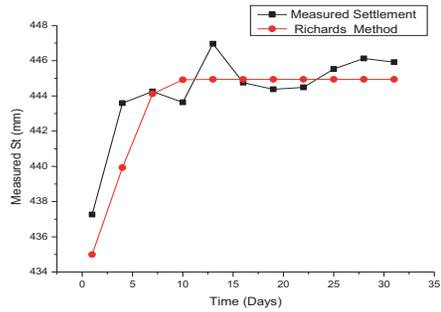
Fig. 3. Measured and predicted settlement values for section K10+850-1
