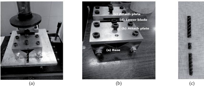
Fig. 2. Double shear test: (a) Instron 3382 Universal Test Machine stand, (b) Double shear testing device, (c) Shear failure of the FRP bar
