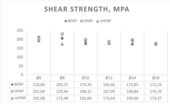
Fig. 5. Shear strength comparison for different bars diameters and types
