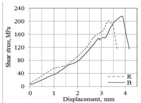
Fig. 3. Shear stress-displacement graph for two different failure modes of HFRP bars with diameter of 14mm.
