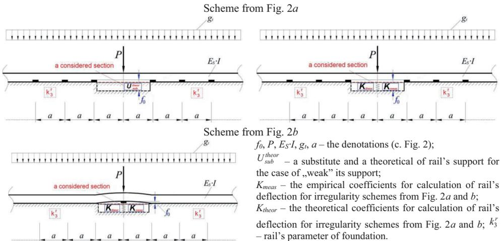
Fig. 5 The exemplary assumed simplified schemes for a analysis of generated irregularities in the track
