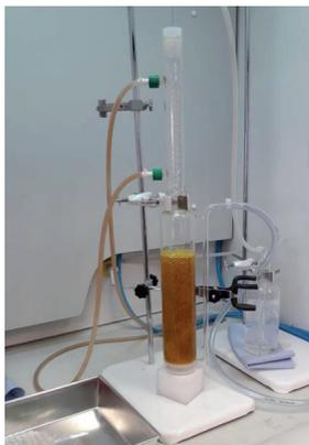
Fig. 1. Ester oxidation reactor
