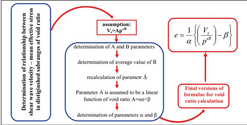
Fig. 6. The procedure for derivation of formula for void ratio calculation
