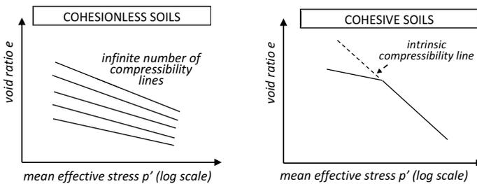
Fig. 1. The differences of compressibility characteristics between cohesive and cohesionless soils curve
