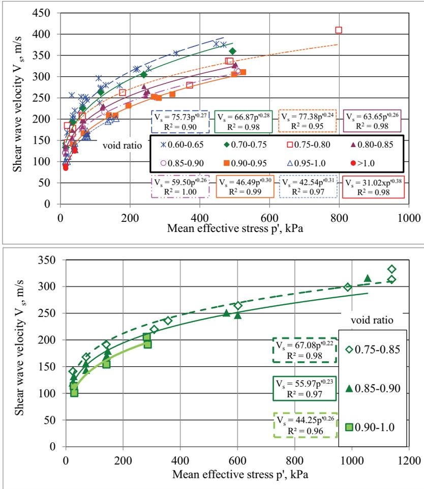
Fig. 5. Power function regressions for  $V_s \sim p'$  relations for each subranges of void ratio of tested materials
