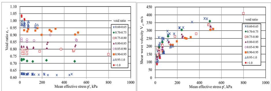
Fig. 3. Shear wave velocity measurements results in various void ratio ranges for fine sand containing 8% of fines
