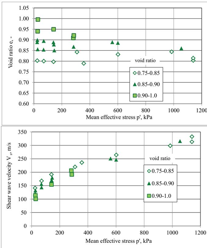
Fig. 4. Shear wave velocity measurements results in various void ratio ranges for fine sand containing 14% of fines
