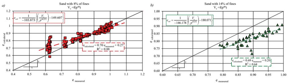
Fig. 7. Comparison of measured and calculated void ratio for fine sand containing 8% (a) and 14% (b) of fines
