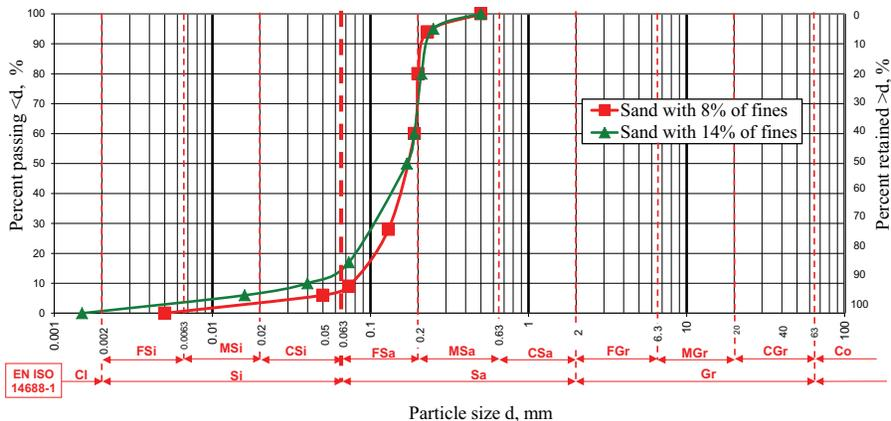
Fig. 2. Grain size distribution of tested materials
