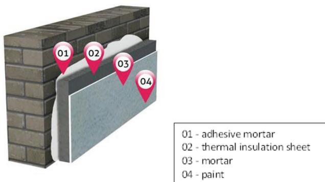
Fig. 1. Layers of the proposed interior thermal insulation application system ([www.eximreno.eu](http://www.eximreno.eu))
