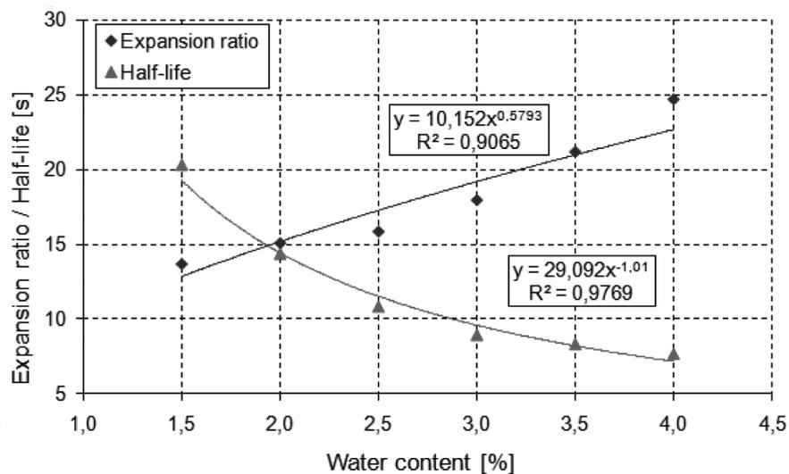
Fig. 1. Characteristics of foamed bitumen for N80 bitumen.
