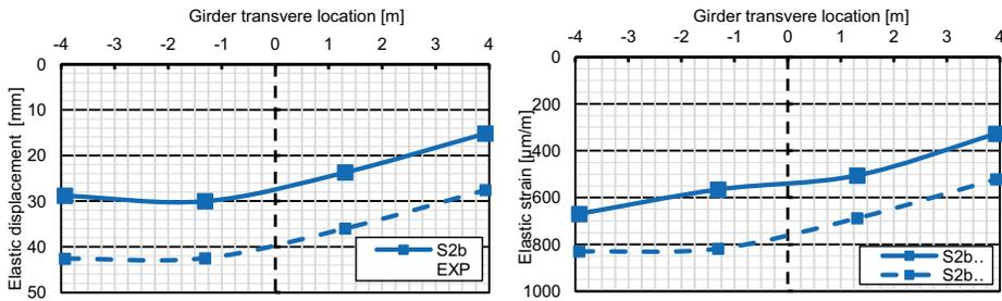
Fig. 7. Transverse distribution of hybrid girder mid-span displacements (left) and strains (right) under the full static load.
