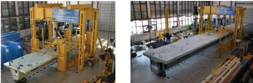
Fig. 4. Research on the structural behaviour of the full-scale bridge girders: a) all-composite GFRP bridge girder; b) hybrid FRP composite – concrete girder.
