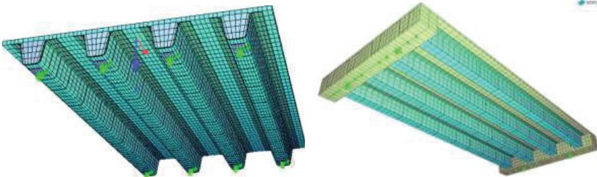
Fig. 3. FE models of the bridge superstructure: a) all-composite bridge; b) hybrid bridge.
