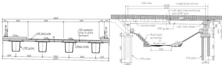
Fig. 2. Cross-section of the hybrid superstructure (left) and side view/longitudinal section (right).
