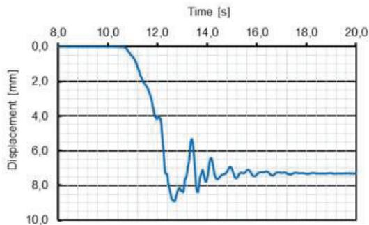
Fig. 6. Maximum deflection in mid-span of the inner girder dynamic scheme (braking on deck).
