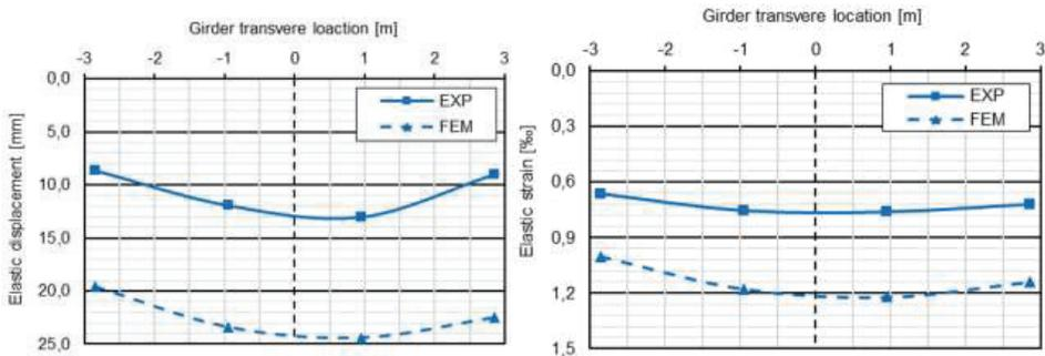
Fig. 5. Transverse distribution of all-composite girder mid-span displacements (left) and strains (right) under the full static load.
