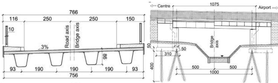
Fig. 1. Cross-section of the all-composite superstructure (left) and side view/longitudinal section (right).
