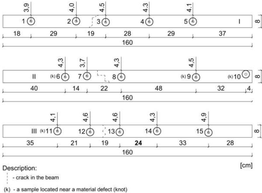
Fig. 1. Distribution scheme of the tested samples.
