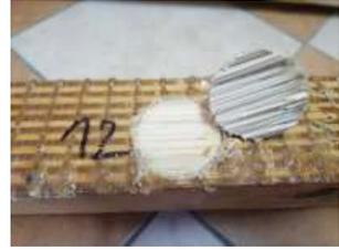
Fig. 6. Cohesive failure in the substrate.
