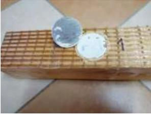
Fig. 4. Adhesive failure between the adhesive layer and the disc
