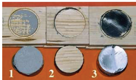
Fig. 3. Damages forms of the tested samples: 1 (cp), 2 (ct), 3 (ap-ad)
