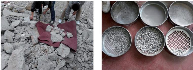
Fig. 1. Selection and screening of waste road concrete
