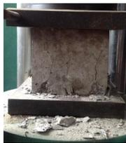
b. w/c ratio 0.55 and aggregate replacement rate 50%
