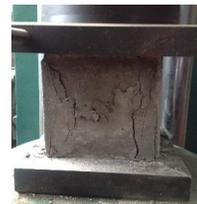
c. w/c ratio 0.61 and aggregate replacement rate 50%
