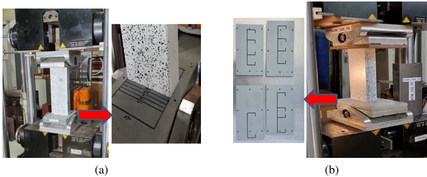
Fig. 4. Experimental stand: eccentricity about minor axis (a) and eccentricity about major axis (b) [19]
