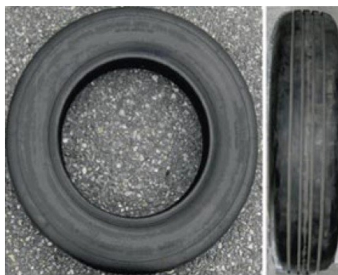
Fig. 4. The test tire PIARC 165 R15 for the SRT-3 [13]
