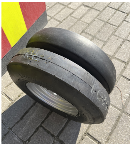
Fig. 6. The test tire for the VF. For comparison, a new tire is shown (bottom) and after 600 km of measurements (top)
