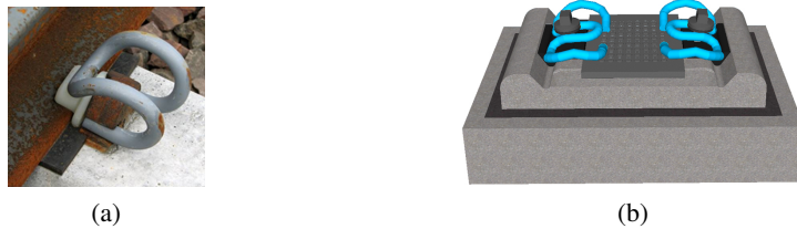
Fig. 16. Illustration principle of classification of rail fastening systems due to the criterion of fixing rail with rail supporting structure – direct rail fastening system: (a) SB fastening system, (b) embedded blocks system with tension clamps type Skl 14 [11]
