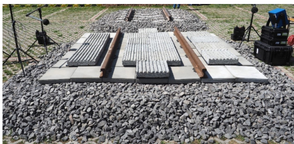
Fig. 27. Prototype sound (noise) absorbing panels made of porous concrete during acoustic tests at the Faculty of Civil Engineering of the Warsaw University of Technology [28]
