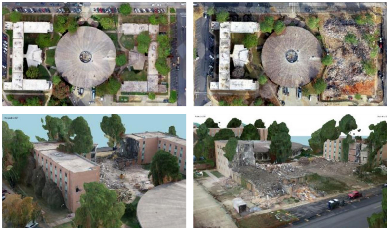
Fig. 6. Orthophoto mosaics and 3D models showcasing progress of works [35]
