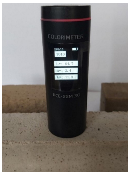
Fig. 4. Determining the colour of the reconstruction mortar using a colourimeter
