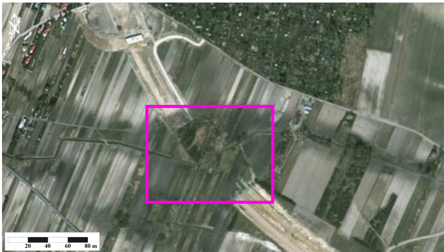
Fig. 1. Unexpected occurrence of thick organic soil layer (violet frame) during construction stage (based on: [8])
