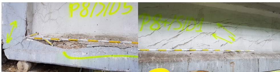
Fig. 2. Web cracks and damage to the pier zones of the WBS beams
