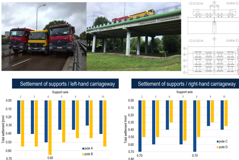
Fig. 4. Settlement of the piers during a static load test on the old bridge
