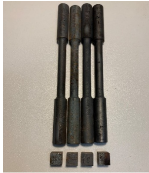
Fig. 3. Selected samples made of the S355J2+N steel grade after simulated fire action
