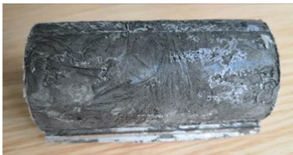
Fig. 4. Soil samples after freezing
