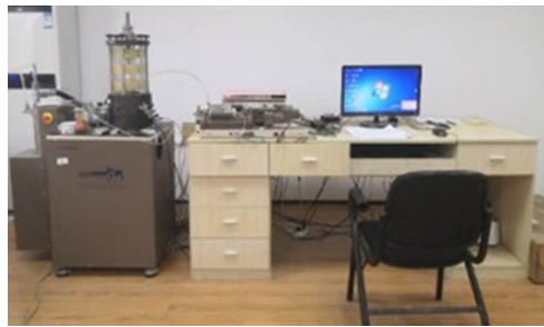
Fig. 1. GDS dynamic triaxial instrument
