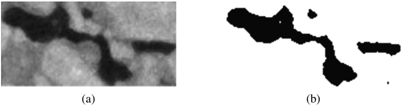
Fig. 7. The CT image of local void in SMA-13 asphalt mixture
