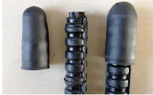
Fig. 18. Protective cap (left), unbonded prestressed tendon (middle), and unbonded tendons of the protective cap (right)
