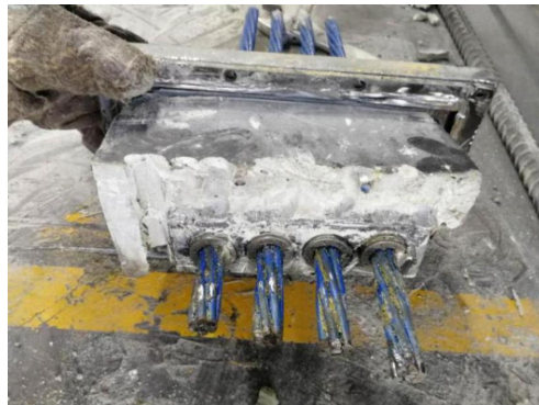
Fig. 19. Seal performance test of epoxy mortar sealing anchorage
