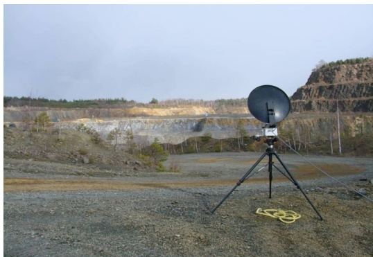
Fig. 12. Position of Doppler radar short time for ignition in quarry
