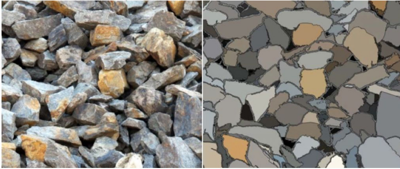
Fig. 4. Land Surveyor measurement: left is cutout of the created orthophotomap and right are detected fragments of the muck-pile [13]
