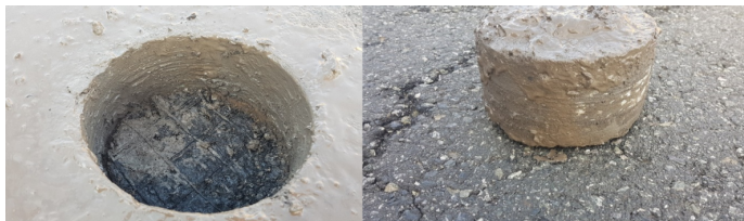
Fig. 1. A glass fiber mesh located under the asphalt layers and an extracted asphalt core (Authors' photo)
