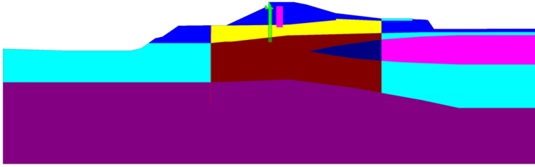
Fig. 8. Seepage and stability calculation model of K26+414 section
