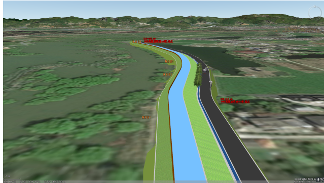
Fig. 7. BIM+GIS data base of West Danger Levee
