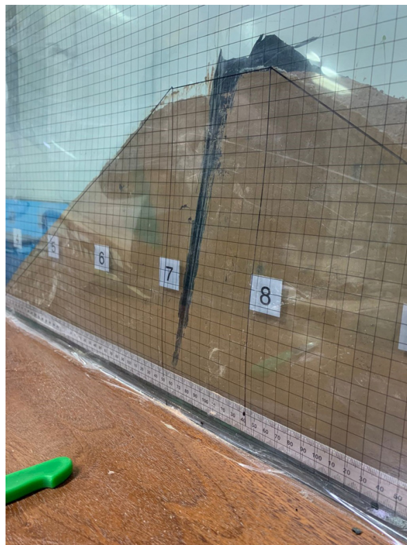
Fig. 8. Insulator in the core of the earthen dam model
