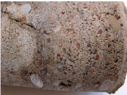
Fig. 6. Porous bottom part of core specimen \phi 100 mm Fig. 7. White drop-stones in the structure of bottom part of core specimen
