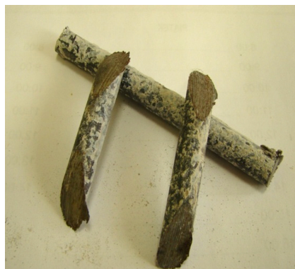
Fig. 9. Carbonation test in the bottom part of core specimen
