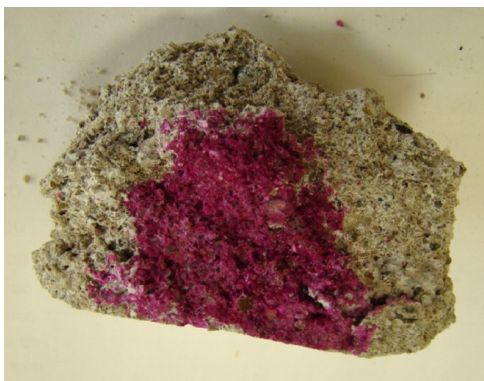
Fig. 8. Carbonation test in the bottom part of core specimen
