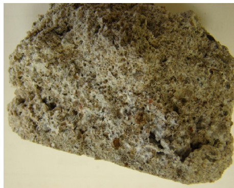
Fig. 6. Porous bottom part of core specimen \phi 100 mm Fig. 7. White drop-stones in the structure of bottom part of core specimen
