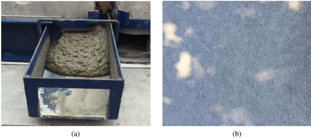
Fig. 11. Effect of 50% sand ratio on the quality of vent concrete; (a) State of vent concrete; (b) Surface quality of filling layer
