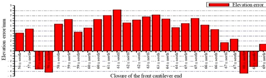
Fig. 22. Elevation error diagram of each cantilever end before closing
