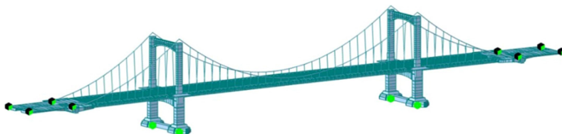
Fig. 4. Finite element model of self-anchored suspension bridge
