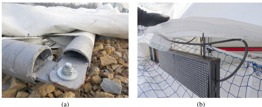
Fig. 7. Elements of fastening and equipment of the pneumatic hall after the disaster: (a) corner connection of the peripheral steel pipe with visible traces of corrosion, (b) elements of equipment attached to the membrane with plastic clamps
