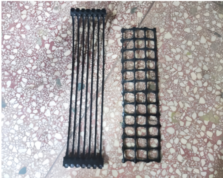
Fig. 2. Geogrid for testing
