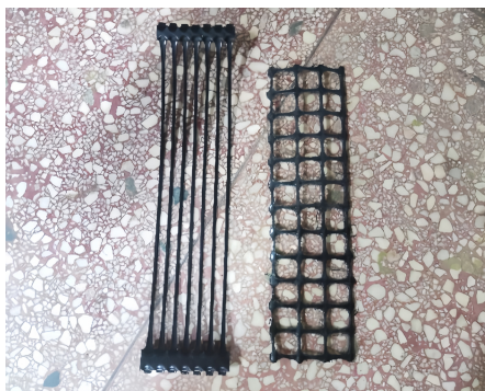
Fig. 2. Geogrid for testing
