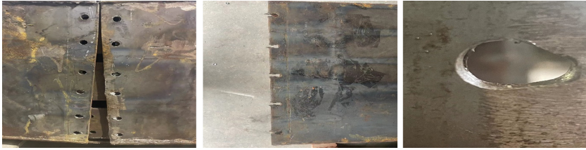
Fig. 19. Photos of mother plates failure
