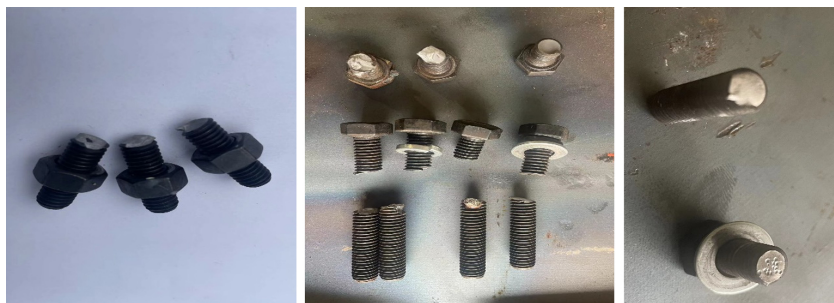
Fig. 18. Photos of bolt failure
