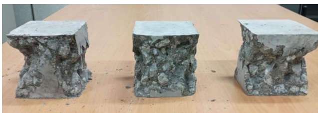
Fig. 5. Pattern of failures for APWP concrete
