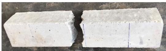
Fig. 7. Pattern of failures for APWP concrete beam
