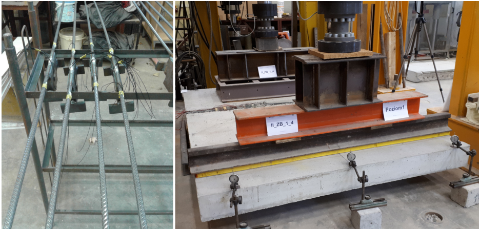
Fig. 3. Balcony connection with glued strain gauges before assembly of reinforcement in set I_ZB_1_1 – without muff on longitudinal reinforcement bars (Stage I) (on the left) and photo of the test stand during research (on the right)
