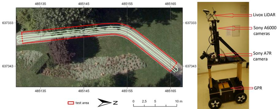
Fig. 2. Test area in Pole Mokotowskie, Warsaw where the measurements were performed (trajectory of measurement showed in green, left side) and platform presentation (right side)
