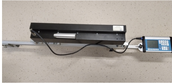
Fig. 3. X-Y profiler measuring system [Photo. J. Kukulski]
