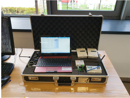
Fig. 3. iBros remote sensors set measuring CO 2
