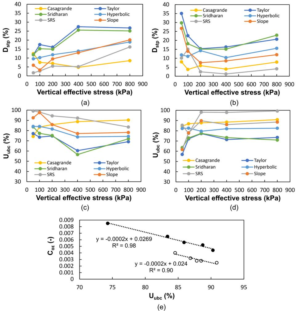
Fig. 7. Soil behaviour at EOP consolidation; (a)  $D_{stp}$  versus  $\sigma'_v$  for Clay 1, (b)  $D_{stp}$  versus  $\sigma'_v$  for Clay 2, (c)  $U_{abc}$  versus  $\sigma'_v$  for Clay 1, (d)  $U_{abc}$  versus  $\sigma'_v$  for Clay 2, (e) relationships between  $c_{\alpha\epsilon}$  and  $U_{abc}$
