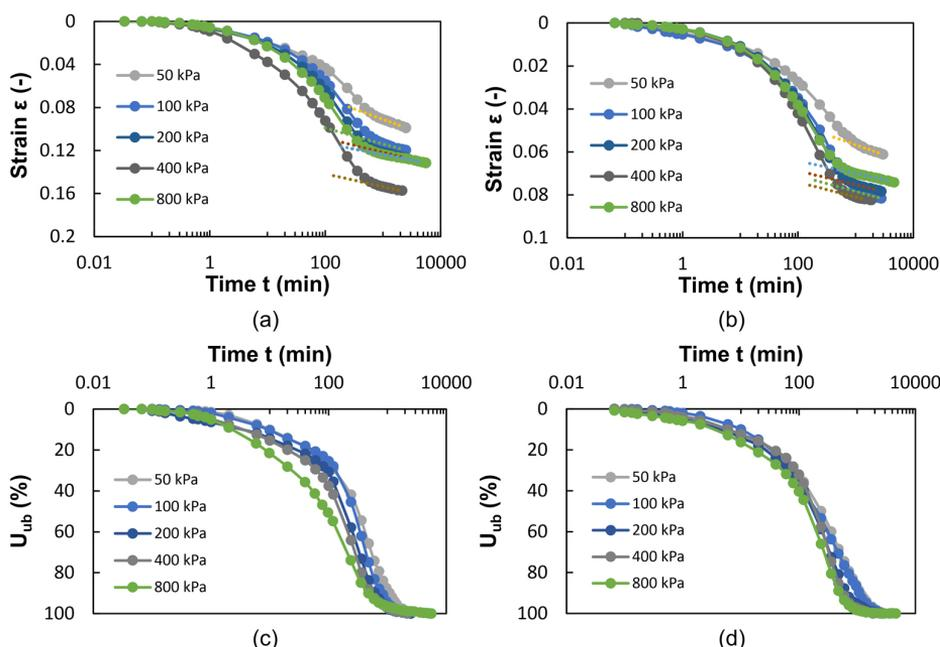
Fig. 4. Consolidation behaviour of soils; (a) vertical strain vs time curves (Clay 1), (b) vertical strain vs time curves (Clay 2), (c) degree of dissipation  $U_{ub}$  vs time curves (Clay 1), (d) degree of dissipation  $U_{ub}$  vs time curves (Clay 2)
