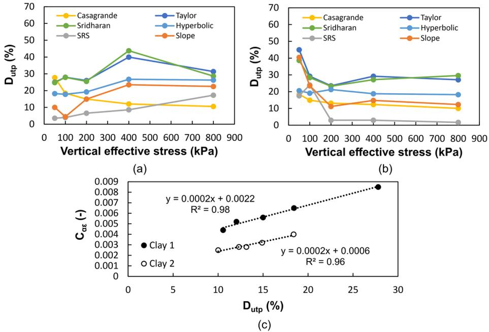
Fig. 6. Magnitude of remaining pore pressure  $D_{otp}$  determined by various methods; (a) Clay 1, (b) Clay 2, (c) relationships between  $c_{\alpha\epsilon}$  and  $D_{otp}$  based on the Casagrande method
