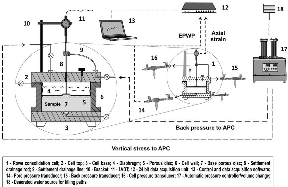
Fig. 1. Schematic of the Rowe cell consolidation set-up
