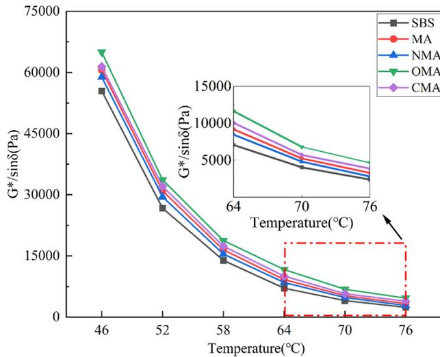
Fig. 3. Rutting factor-temperature diagram of different asphalt samples
