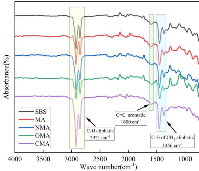
Fig. 2. FTIR spectra of different asphalt samples
