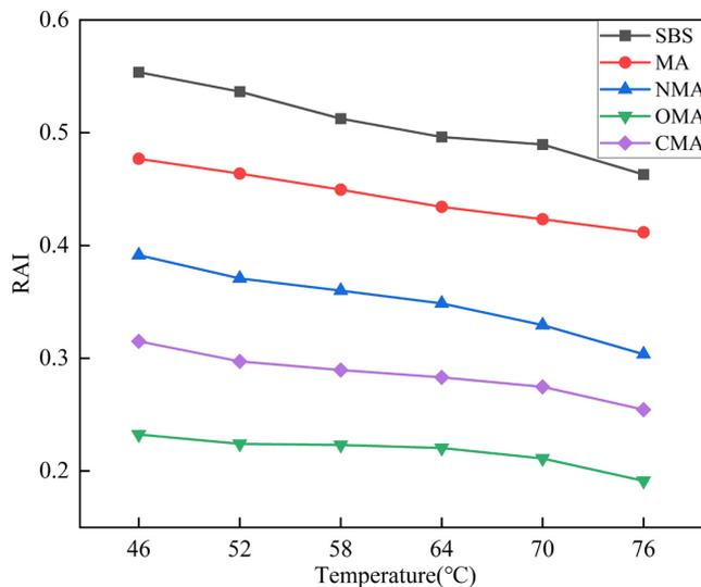
Fig. 10. Short-term aging rutting factor index of different asphalt samples
