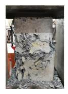
Fig. 7. Typical failure mode of specimen with  $s_h = 52$  mm failed at  $\varepsilon = 0.05$
