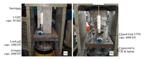
Fig. 4. Test setup: (a) front view; (b) back view.
