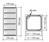
Fig. 2. Details of test specimen
