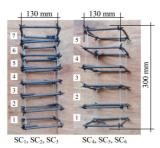
Fig. 3. Details of test specimen stirrups:  $SC_1$ - $SC_3$ ,  $s_h$  = 36 mm;  $SC_4$ - $SC_6$ ,  $s_h$  = 52 mm
