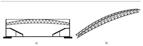
Fig. 1. a) Cross-section through the considered steel hall, b) the view of the spatial truss girder.
