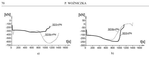
Fig. 6. Comparison between SD3+PN and SD3b+PN. Axial force: a) for the top chord, b) for the diagonal.
