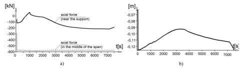
Fig. 8. Case SD3-ih+PN+izo: a) axial force (top chord), b) vertical displacements in the middle of the span.
