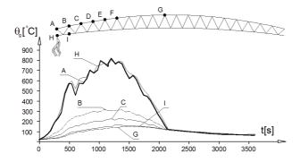
Fig. 4. Fire curves received for thermocouples arranged along the span of the truss (case L1). Results for D,E, and F are not presented in order to provide clearness of the figure. D,E,F fire curves are contained between C and G.
