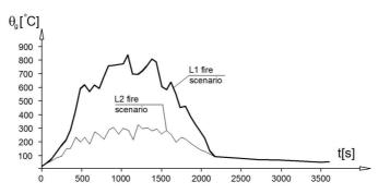
Fig. 3. Comparison of temperature measured at the level of the lower chord. Fire scenarios L1 and L2.
